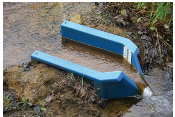
Portable Weir on a Small Stream
