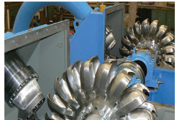
Dual Pelton Turbines
