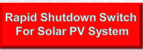
Sign located next to the rapid shutdown disconnect (and must be reflective)
